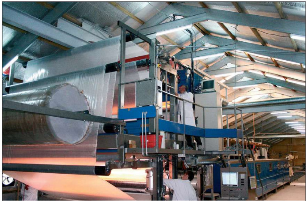
The huge laminating machine carries out all the work to apply Utex to the Mylar film, positions the threads, sticks them together and heats it up
