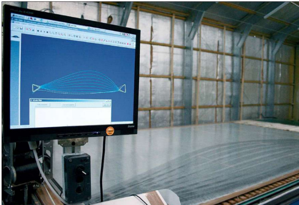
The software directs the arm, which positions the fibres on the Utex-Mylar backing.
